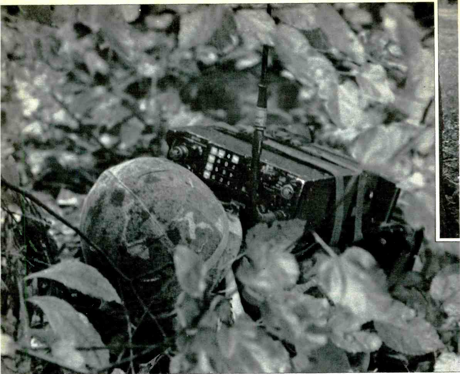
SINCARS can handle both voice and data. It has a built-in capability to handle data at a rate of 16 kilobits. With the available data rate adaptor, it can also handle standard data rates from 75 to 4800 baud. (US Army photo)
