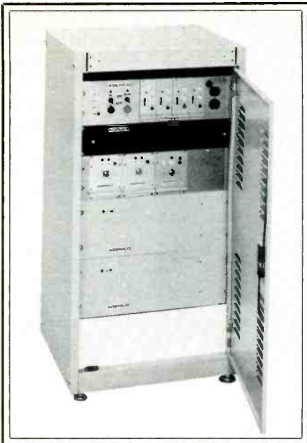
The transmitter/receiver console for a central station.
